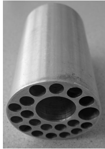
Figure 4.10: Photo of Hannink’s sample: twenty tube resonators with different radii and lengths.
