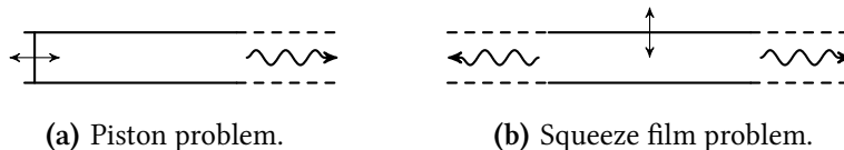
Figure 3.11: Two extremes of fluid structure interaction problems. In ‘piston’ problems, the viscous effects at the piston can be neglected. In ‘squeeze film’ problems, viscous effects at the moving structure are important and cannot be neglected, but the errors remain small.
